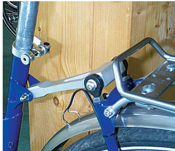
igubal® rod end bearings in the spring loaded rear axle rocker of a bicycle
