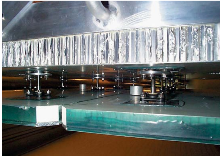
igubal® flange bearing in the reflector adjustment of the telescope
