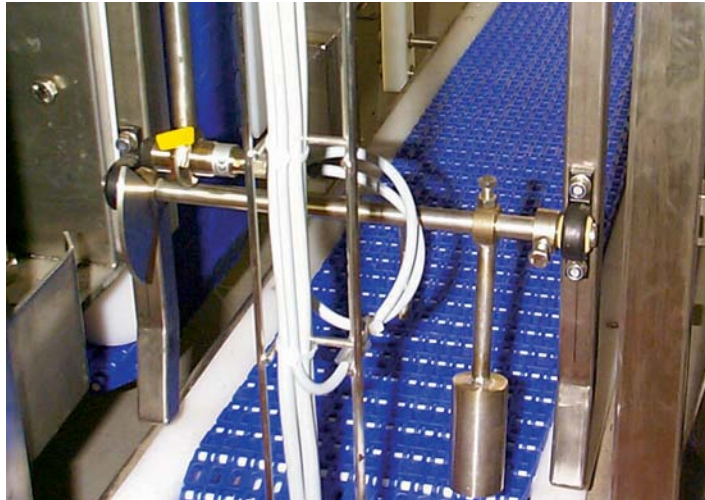
igubal® pillow block bearings in a conveyor system
