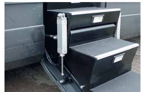
igubal® rod end bearings in the cylinder-controlled steps of an RV
