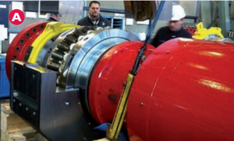
Cooper double row 780mm bore split tapered roller bearing on a link-spindle for a steel making plant.
