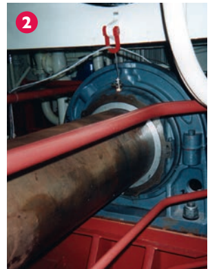
2. A typical installation of a Cooper BCP on a propulsion shafting application.
